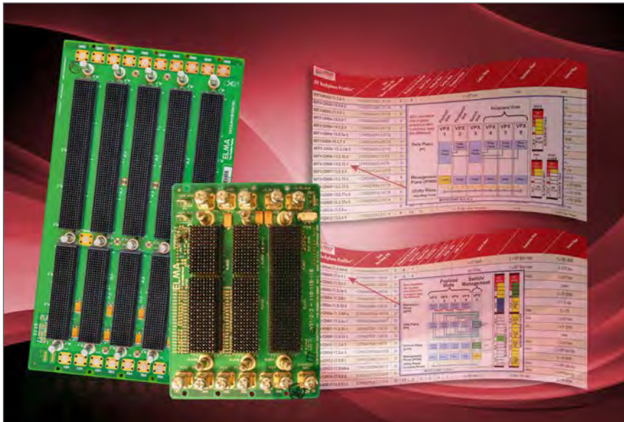
Figure 1 | Being part of the OpenVPX steering and marketing committees has enabled Elma to offer deeper resources, such as these backplane profiles that assist users in the development of OpenVPX-based systems.
