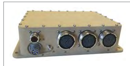
Figure 1 | The DuraDBH-672 Digital Beachhead Gigabit Ethernet switch and vetronics computer subsystem addresses the U.S. Army's ground-vehicle GPS modernization efforts.
