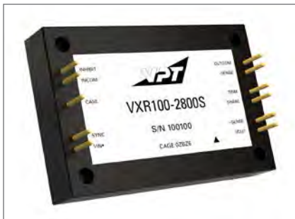
Figure 2 | The VXR100-2800S from VPT Inc. is aimed at use in applications such as military ground vehicles, commercial and military aircraft, and unmanned aerial and ground systems.
